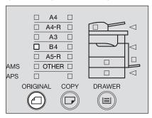
4 Press the [COPY] button several times until the lamp of the desired paper size is lit.
